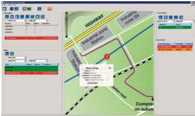
*Omnisens Map gives a graphical representation of the location of events which prompt an alert. The asset route data is provided by the client and integrated into Cobra by Omnisens. The temperature profiles are also available for analysis.*
